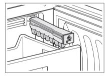
Pull out the tap. Fill with water to the limit indicated "MAX".
